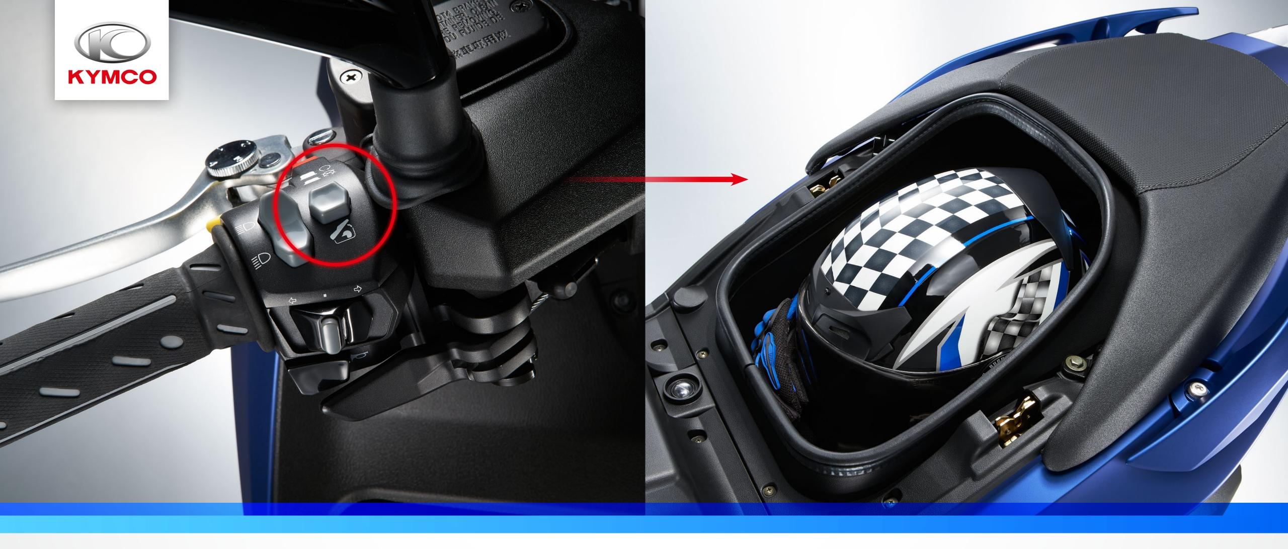
The unique two-stage seat opening design that could be operated by pushing the left side button of handlebar or key makes access to the under-seat compartment easier than ever.
