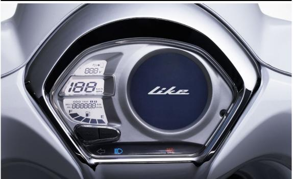
• Digital Clock • Speed • Battery Voltage • Fuel Level • USB Charging Port Status
